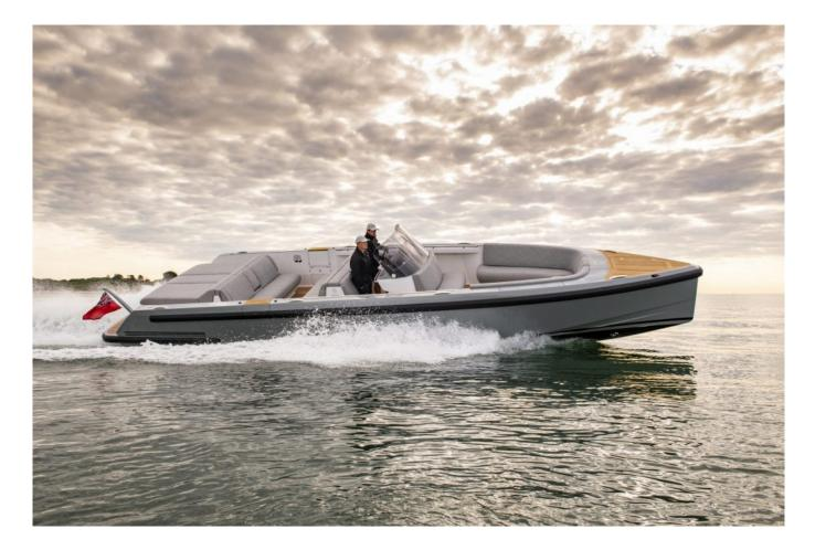
The 11.6m tender has an impressive top speed in excess of 40 knots, with power derived from a pair of Yanmar 8LV 370hp engines.
