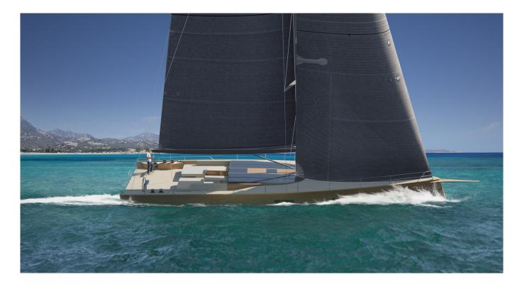
Minimising local emissions was key to the design brief, and the choice of a 30kW electric engine which also has the ability to hydrogenerate through her free-wheeling propeller while sailing, reduces emissions to virtually nil, with no fossil fuels being burned and no noise pollution.
