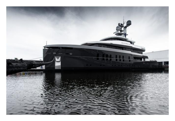
Shinkai, which means 'deep sea' in Japanese, is set to embark on many far-reaching expeditions in the coming years. These will include both the northwest and northeast passages. The vessel's steel hull has been built to ice-class standards to ensure she can weather the extreme conditions of such voyages. Additionally, for the first time on a yacht of this size, a
